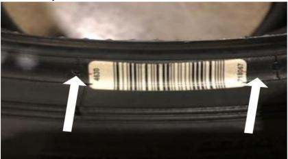
**3.4 Drill two 13mm holes** in the tire sidewall above the bar code label. Take a picture of the holes, including the barcode label.
