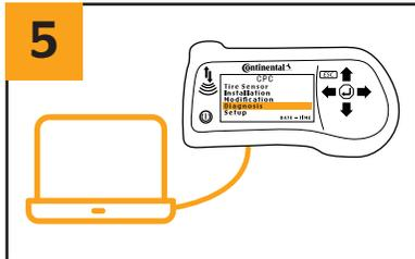
Plug the provided USB cable into the HHT and plug the other end into your computer. If you have not programmed sensors with the HHT, skip to step 11.
