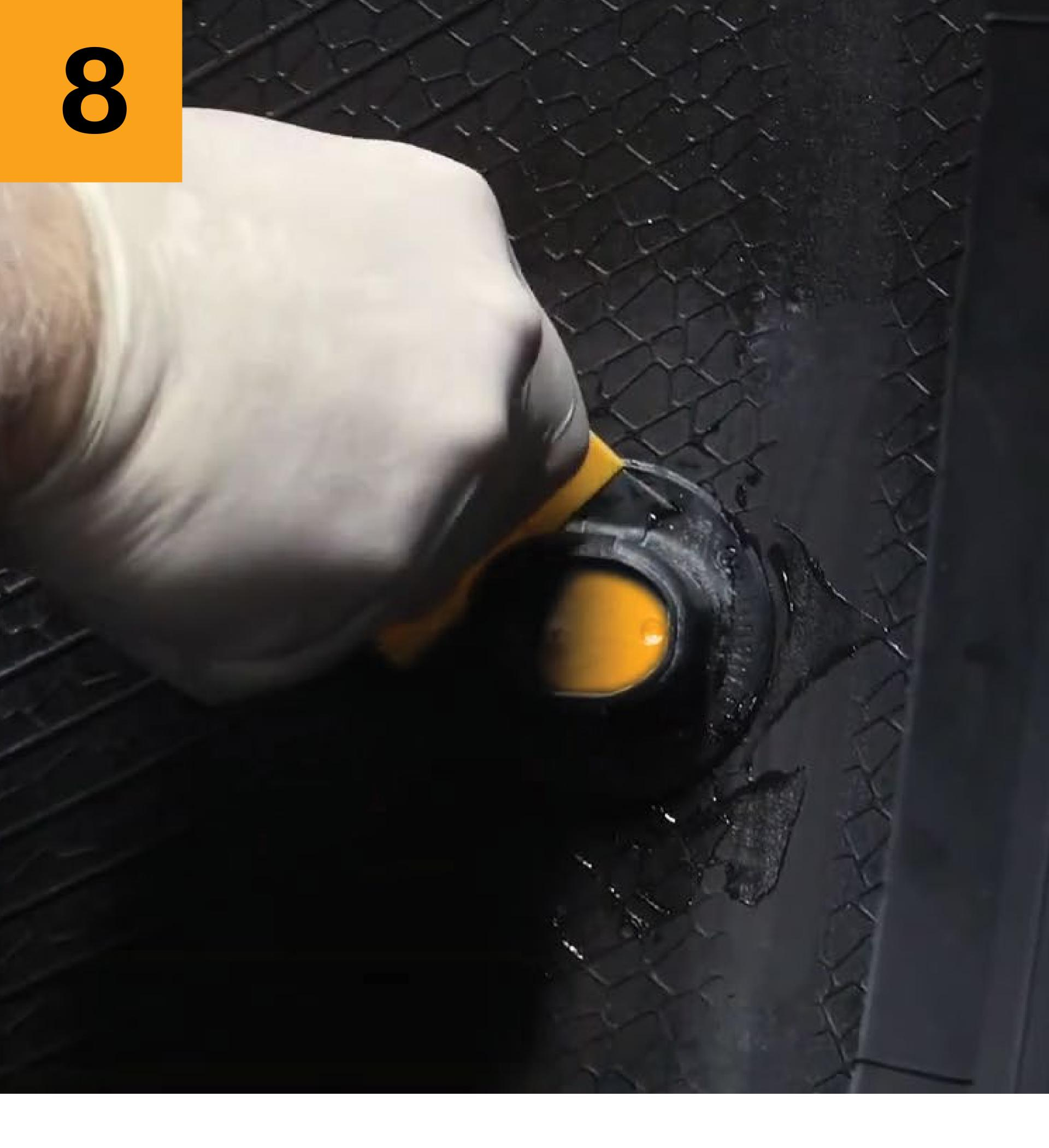
Remove the mounting tool and use the spatula to push against the outside edge of the boot, ensuring a secure fit.
