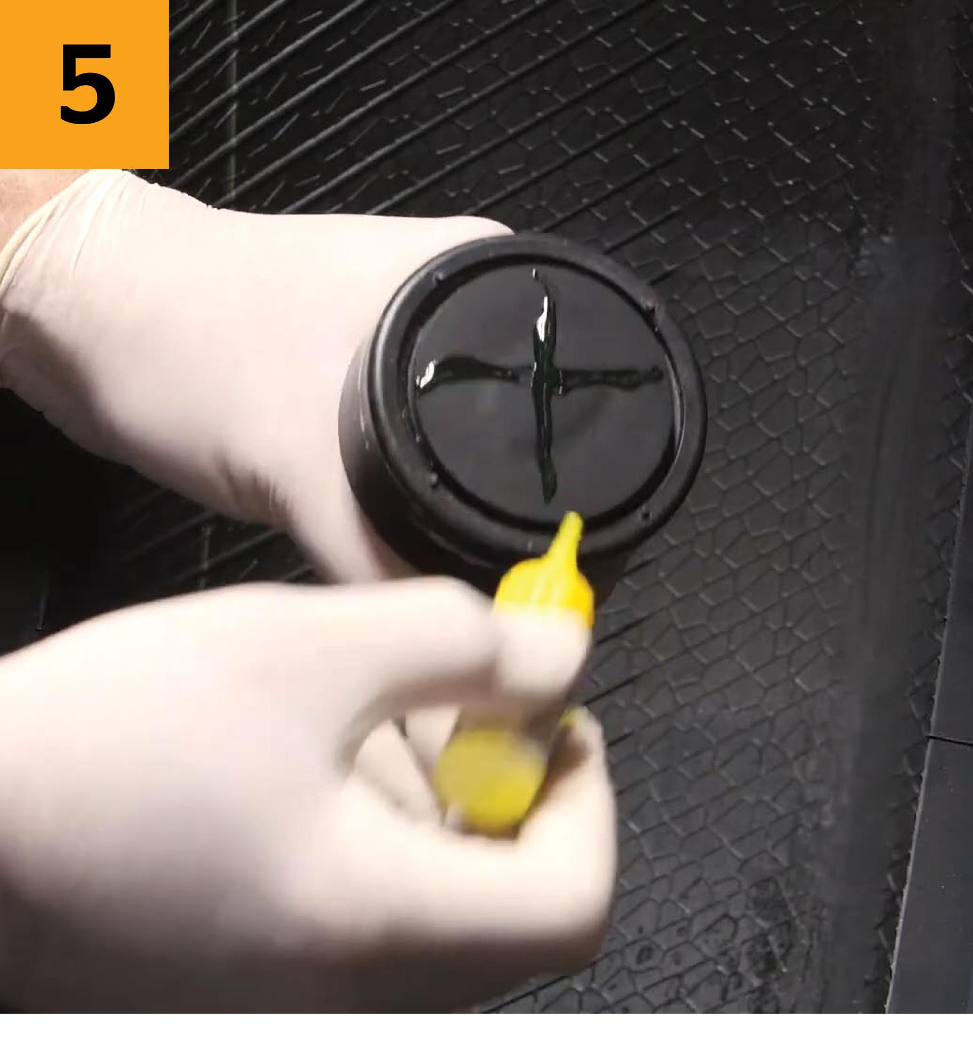
Place glue on the bottom of the boot in an "X" pattern and use the spatula tool to spread the glue around the entire bottom of the boot.
