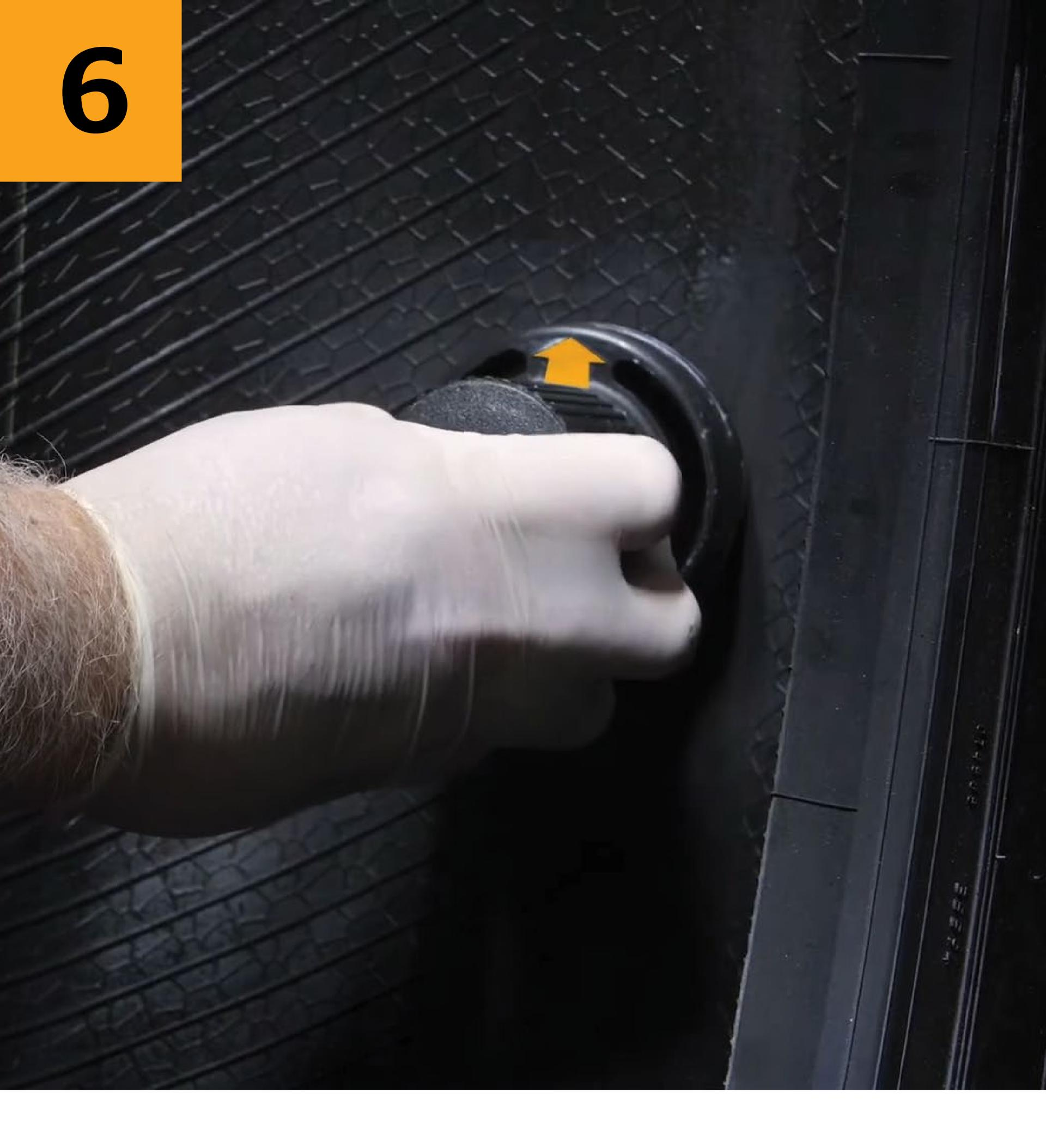
Press the mounting tool with the arrows facing the direction of tire rotation onto the tire where you previously buffed in step 2.
