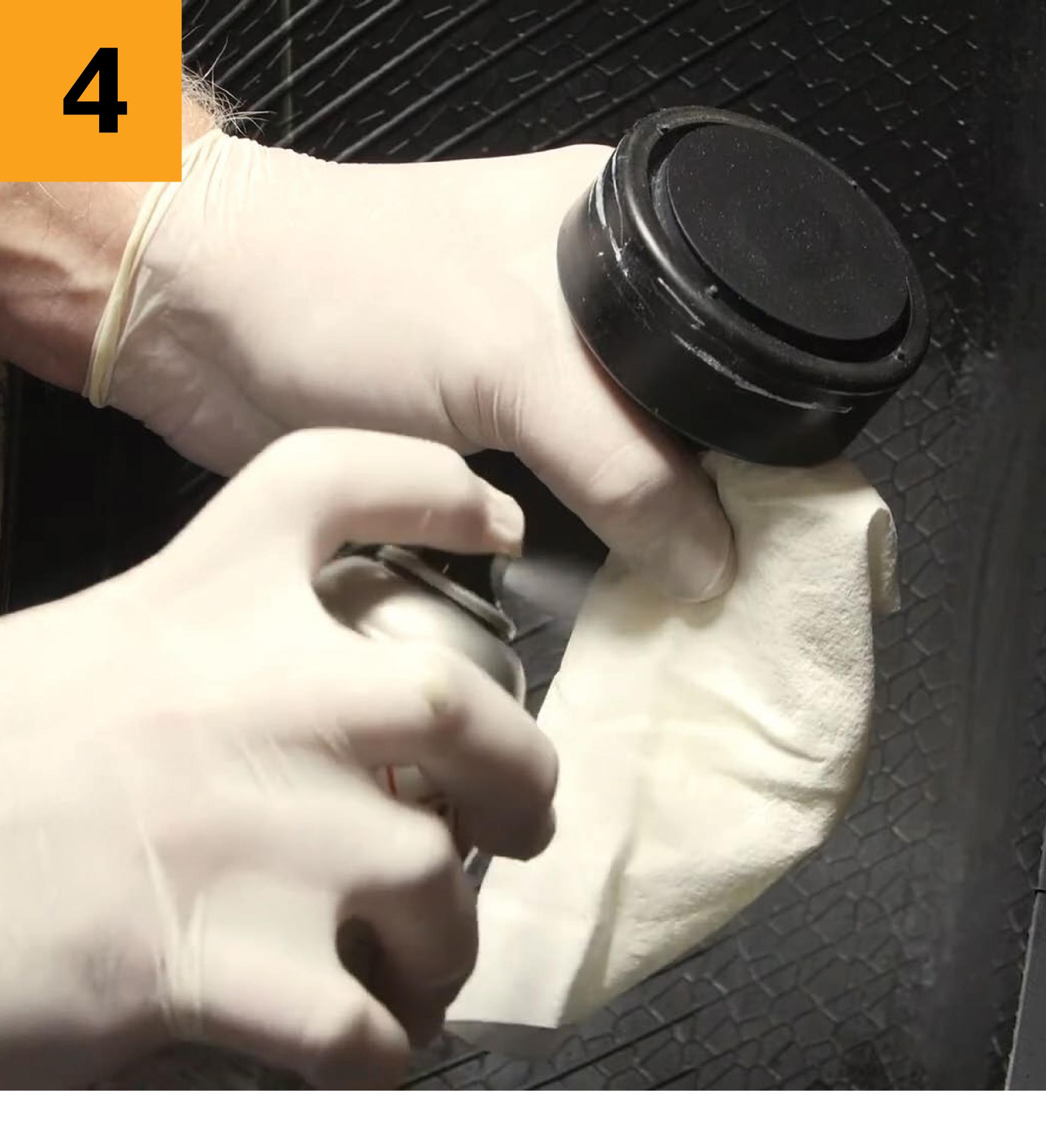
Insert the tire sensor in the boot and place inside of the mounting tool. Clean the bottom of the sensor boot with buff and a towel 2x to remove contaminants from the boot base.
