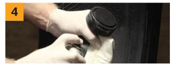
Insert the tire sensor in the boot and place inside of the mounting tool. Clean the bottom of the sensor boot with buff and a towel 2x to remove contaminants from the boot base.
