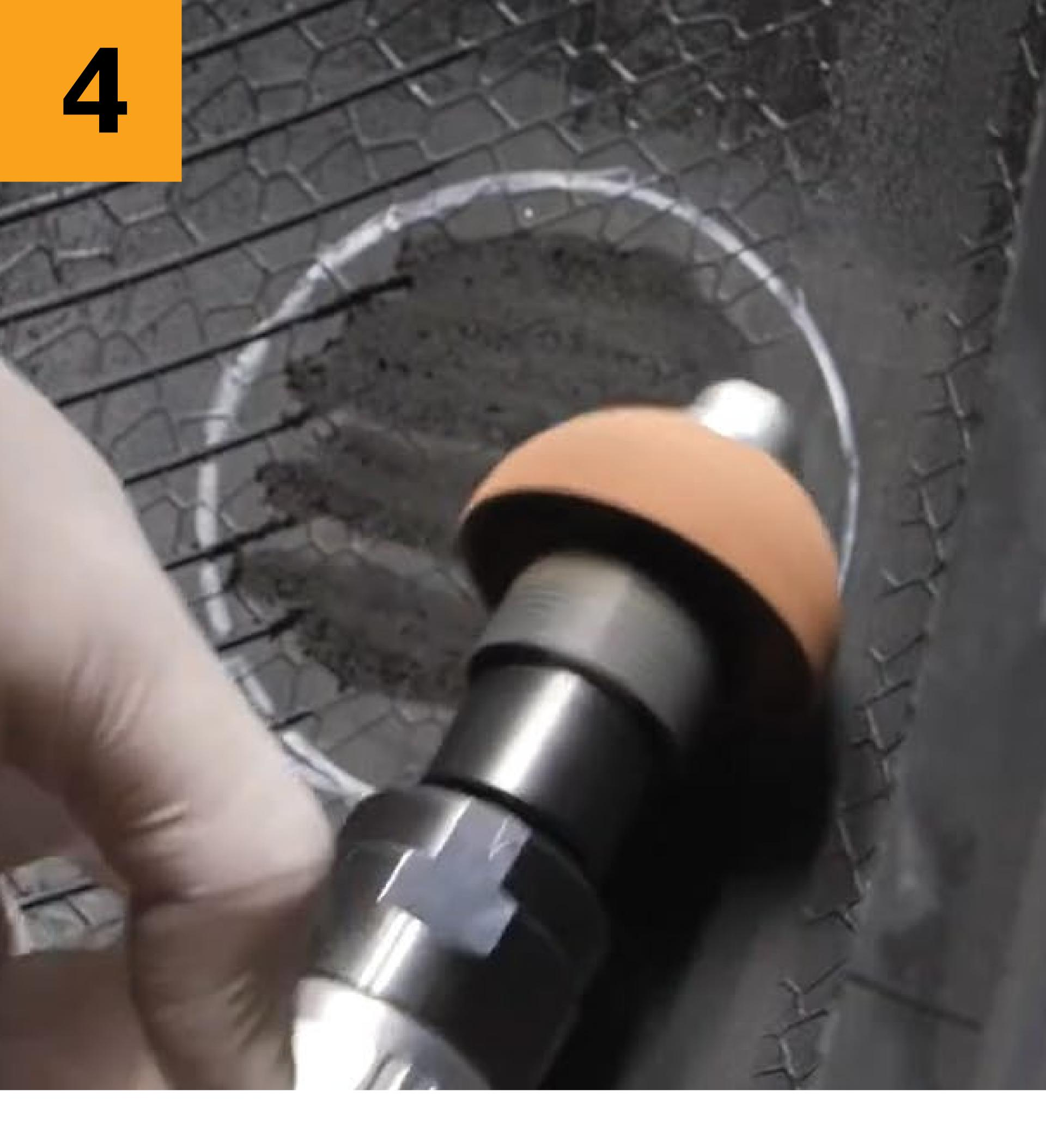
With a low speed buffer and 36 grit buffing bell, use light and constant movement to buff the area inside the chalk.
