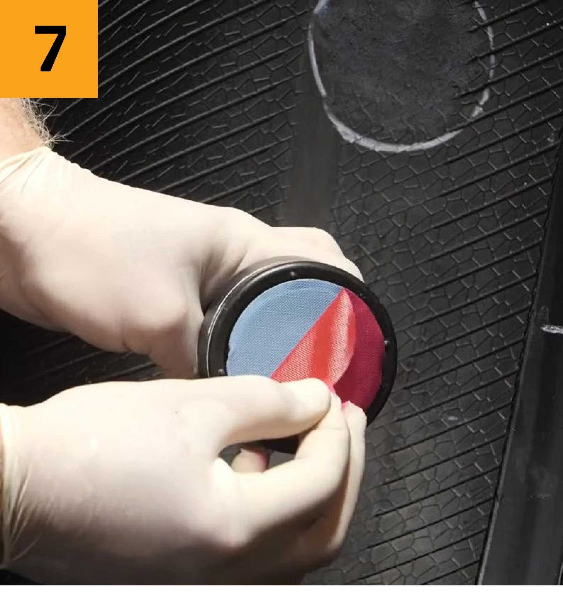
Insert the tire sensor in the boot with REMA patch applied to the bottom, and place inside of the mounting tool. You can now remove the adhesive covering.
