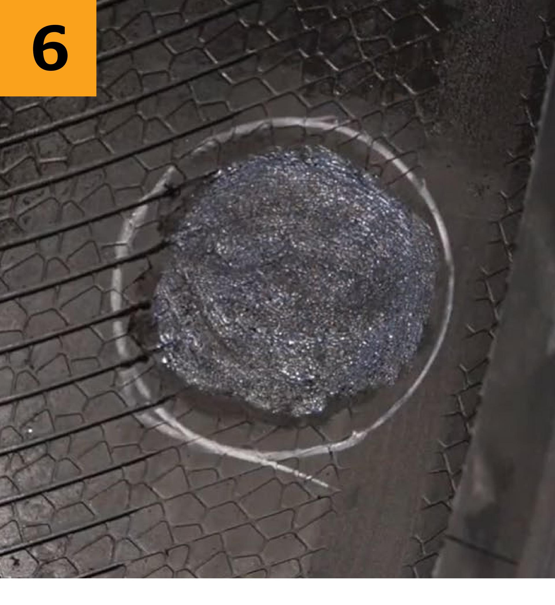
Apply REMA cement using a swirling motion until there is a thin, even coat. Cover the area until it appears to be dry.
