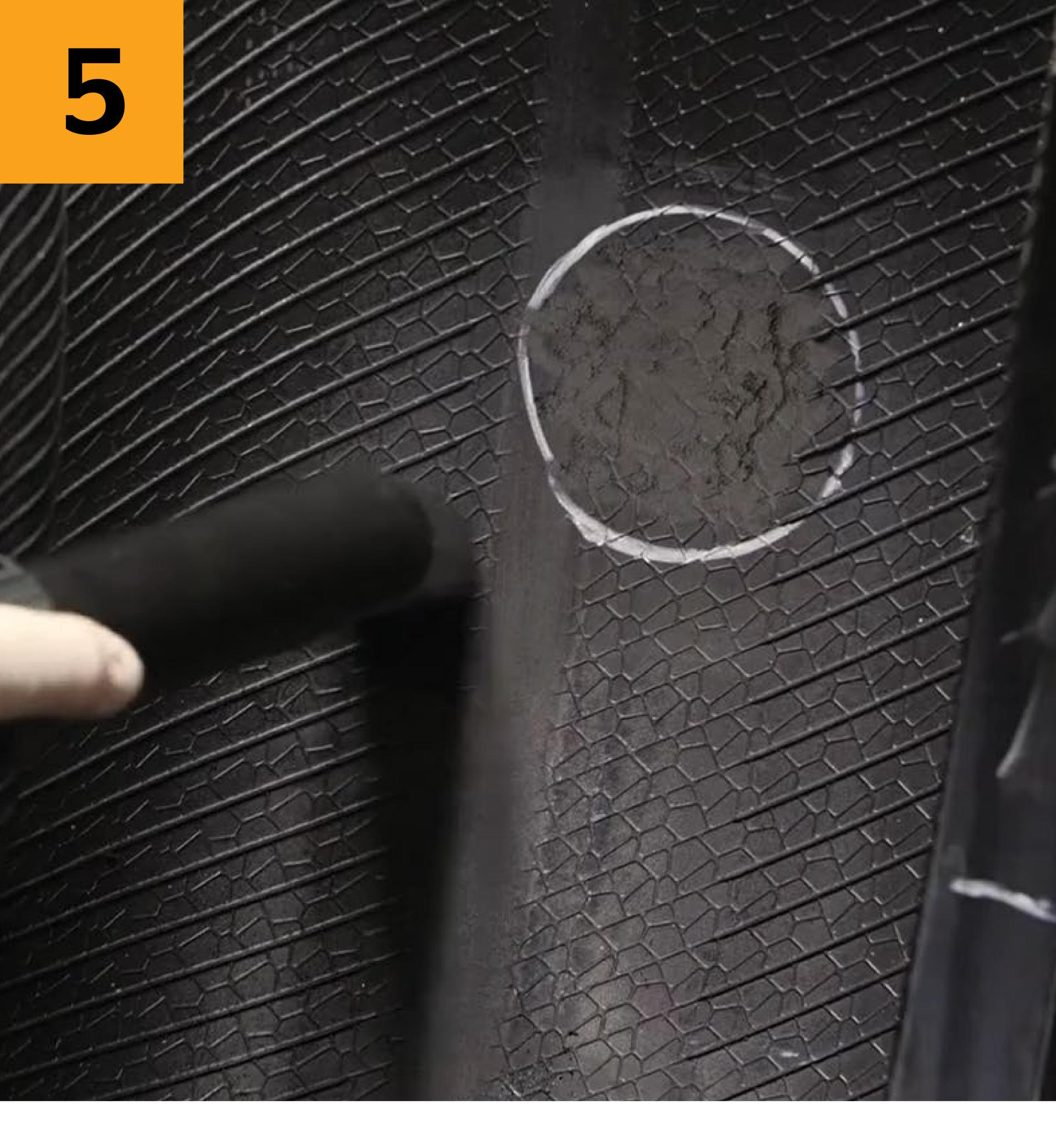
Using a dedicated brass brush clean the buffed area, being careful not to contaminate with the area outside of the chalk. Use a vacuum to clean up any other debris outside of the chalk.
