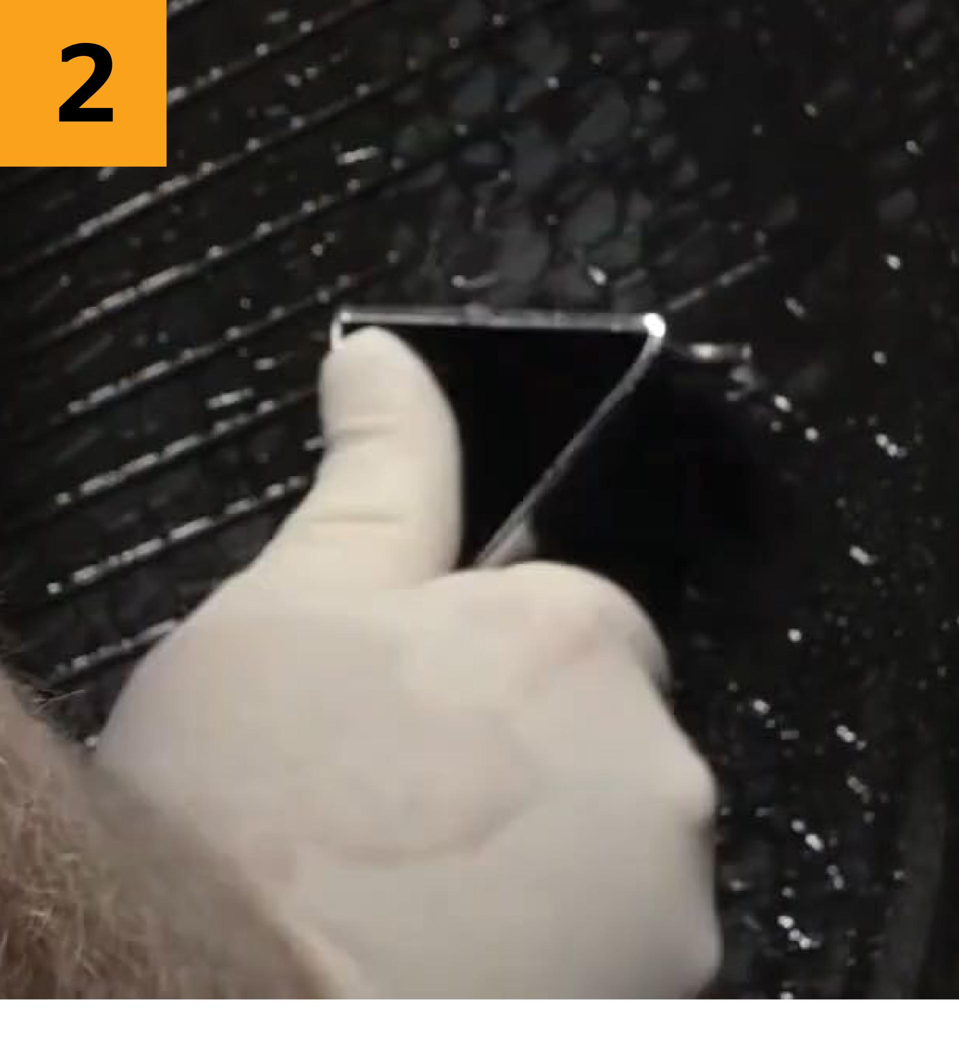
Clean the inner liner of the tire with the handheld scraper tool to smooth out the surface. Spray and scrape 3x - once up and down, once diagonally left, once diagonally right to ensure a wax-free surface.
