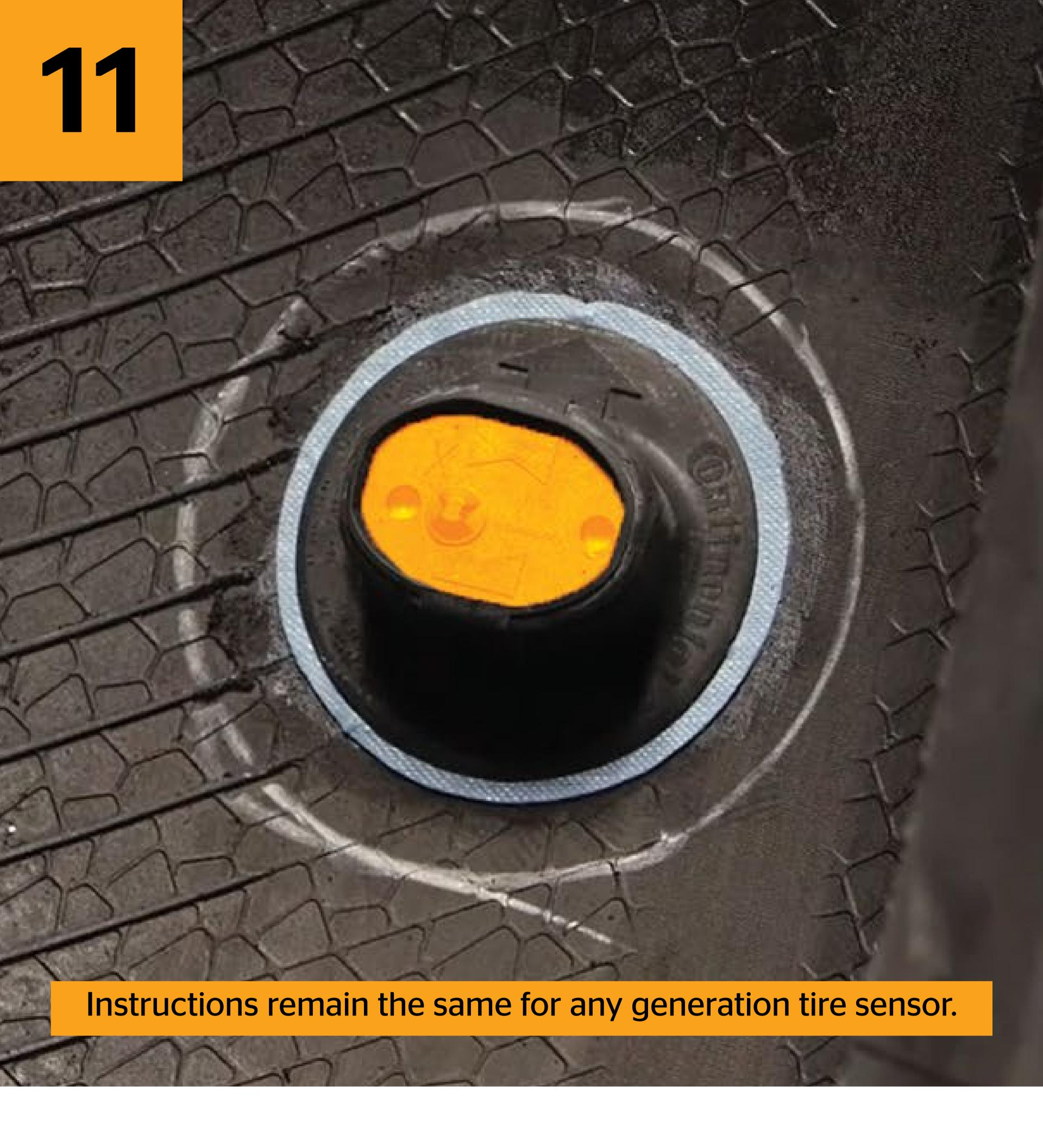
With your hand, gently wiggle/pull the sensor to confirm a secure installation.
