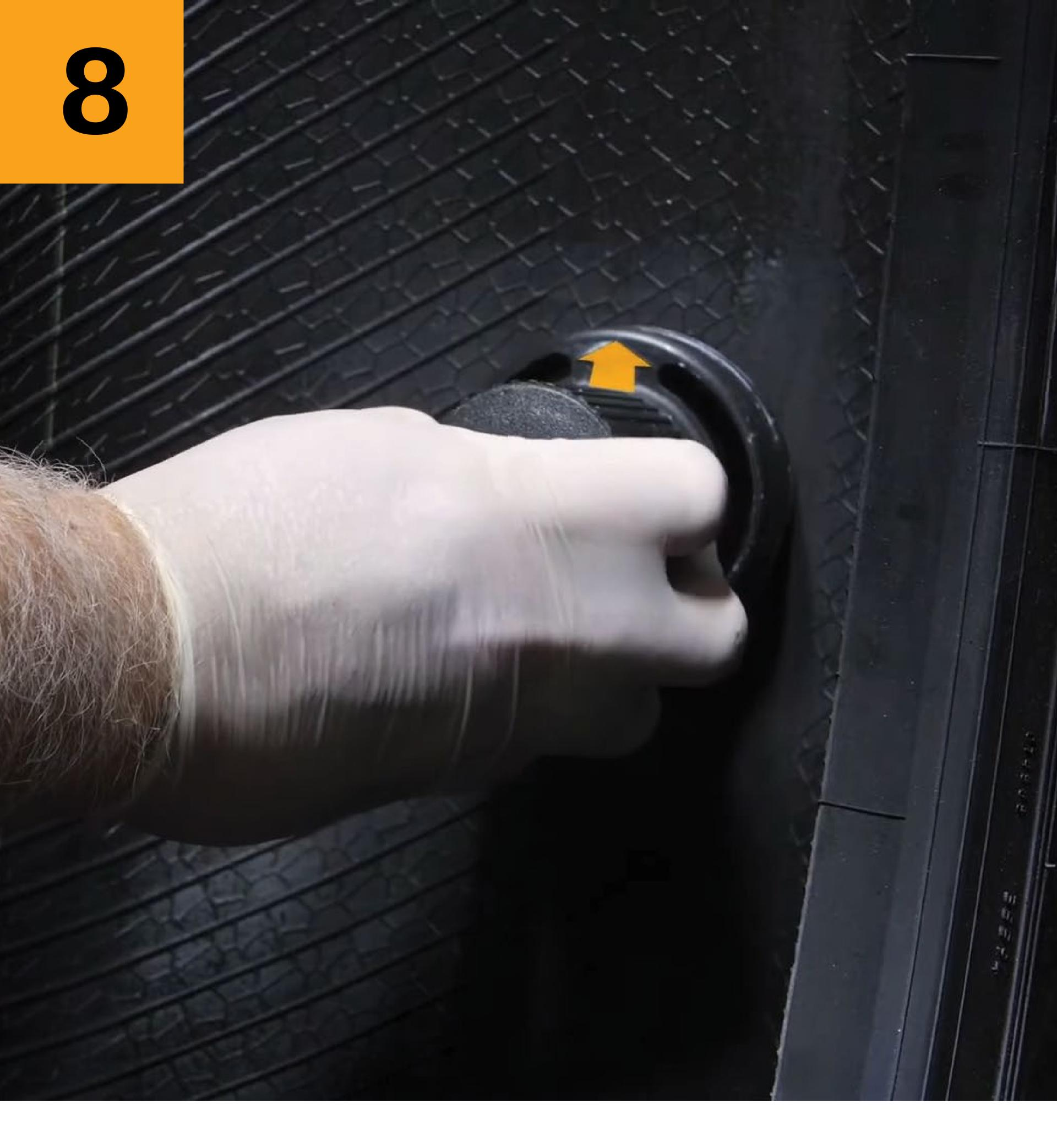
Press the mounting tool with the arrows facing the direction of tire rotation onto the tire where you previously applied the cement.
