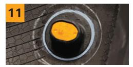
With your hand, gently wiggle/pull the sensor to confirm a secure installation. Sensor installation is complete.
