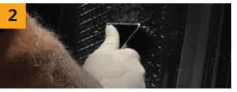
Clean the inner liner of the tire with the handheld scraper tool to smooth out the surface. Spray and scrape 3x - once up and down, once diagonally left, once diagonally right to ensure a wax-free surface.
