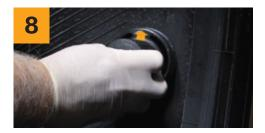
Press the mounting tool with the arrows facing the direction of tire rotation onto the tire where you previously applied the cement.
