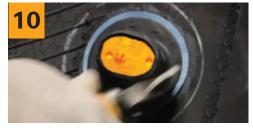
Remove any trapped air around the edges using the roller & stitcher.
