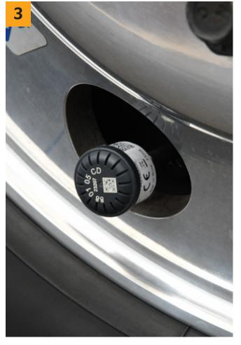
Once the Valve Cap Sensor has been attached, you can begin programming the sensors using the HHT. (See Program Valve Cap Sensor Guide)
