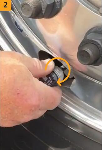
Screw in the Valve Cap Sensor to the valve stem until you hear a brief hiss, indicating it is sealed. Turn the Valve Cap Sensor an additional  $\frac{1}{4}$  -  $\frac{1}{2}$  turn to completely seal the sensor to the stem.
