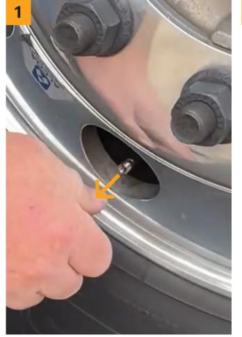
Remove all valve caps from the vehicle's tires and check that they have the correct tire pressures. Adjust tire pressures if necessary.
